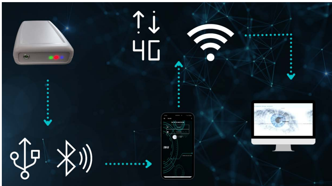
Figure 1. Operation of the Control System. The stimulation devices connect via Bluetooth or USB to the mobile application, which will transmit data via Wi-Fi or 4G network to the server.
